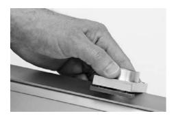
Drill hole using conical drill or drilling tool.
